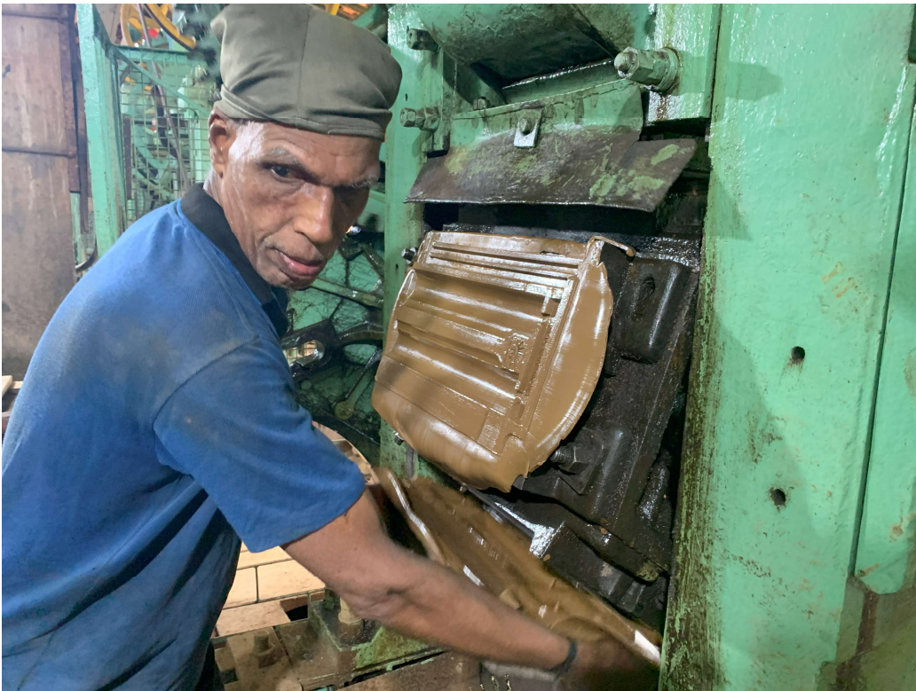
Operator operating with the molding machine at Albuquerque Tile factory, Mangalore
